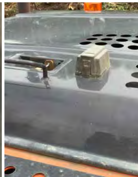
1336-BLK Shown fitted to construction equipment, with supplied rubber cover installed.
