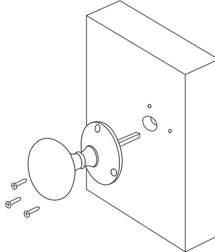
4. Insert the spindle into one handle/knob.
