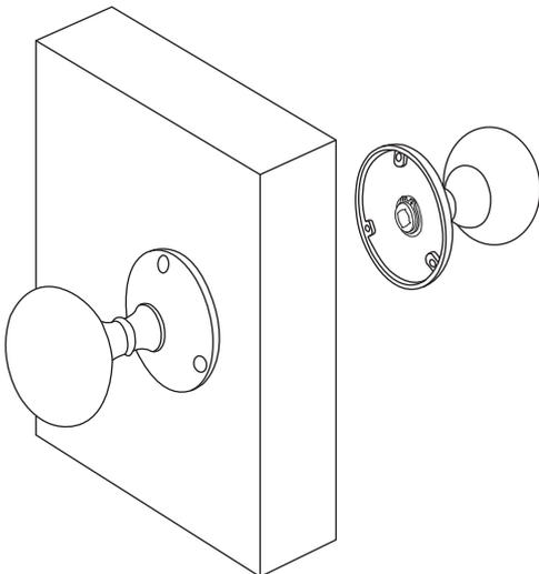
7. Slide the handle/knob on the opposite side of the door onto the spindle ensuring that it sits straight on the door face.
