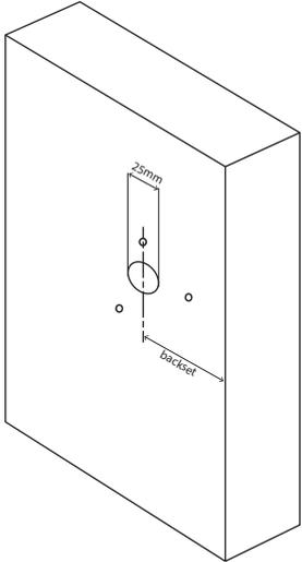
1. Establish the height and position for the handles/knobs on the door.
