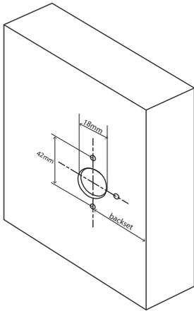
1. Establish the height and position for the handle on the door.
