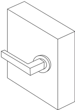
4. Screw the rose cover onto the handle and tighten the grub screw on the side of the lever onto the spindle. For the square rose (Futura Elite) press on the rose cover and tighten the grub screw on the side of the rose.
