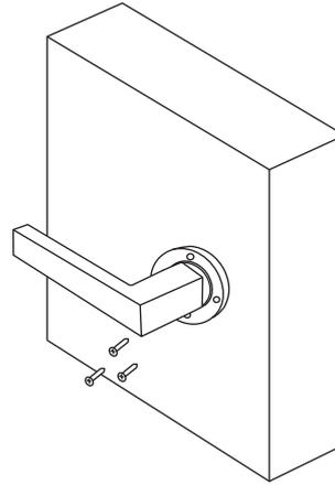
3. Install the handle by screwing the base plate to the door with the wood screws provided.
