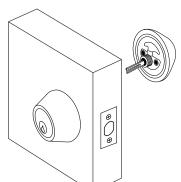
8. Press the internal cylinder/turn flush against the opposite side of the door, ensuring the keyhole/turn is pointing down. For the cylinder ensure the spindle is being inserted through the deadbolt vertically. For the turn the slot for the spindle will be in horizontal position to be able to fit the spindle of the external cylinder. Fasten the cylinder/turn with the screws provided.
