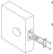
5. Insert the deadbolt, scribe around the faceplate, remove, then chisel out a 4mm recess to enable the faceplate to sit flush with the door edge.
