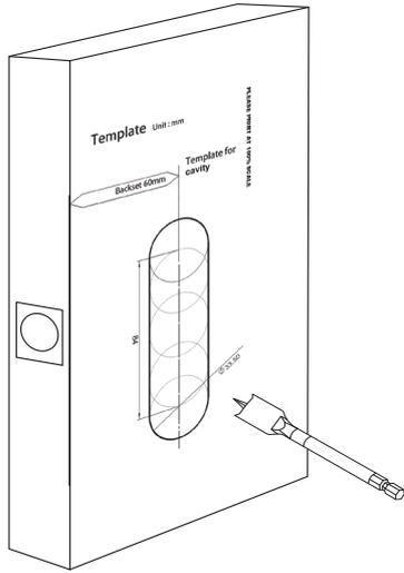
1. Place the template where indicated on the door, lining up the 60mm backset vertical line with the edge of the door.
