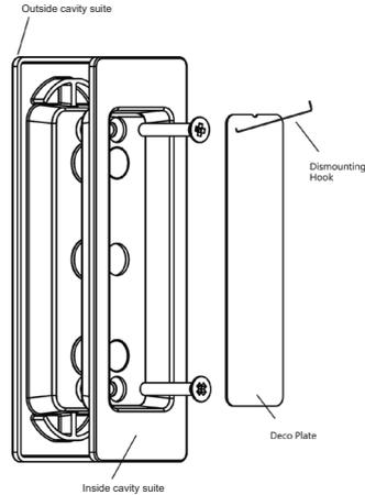
5. Insert the outside flush pull into the cavity in the door face, then insert the inside flush pull and tighten the bolts. Trim the bolts to the correct length if necessary.
