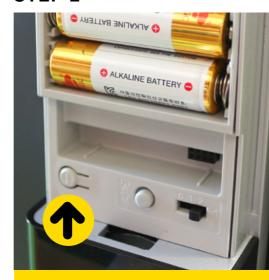
With the door open, push the (I) button located to the left of the three buttons, below the batteries.
