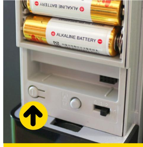
With the door open, push the ( I ) button located to the left of the three buttons, below the batteries.
