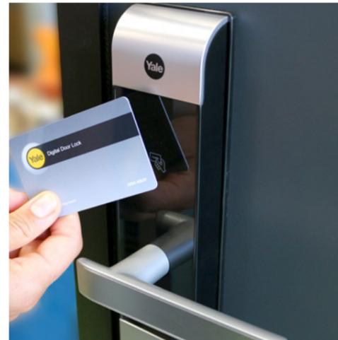
4 cards are supplied with the lock. To register cards, first push the ( I ) button, then present cards to the keypad, one by one. As each card is registered, a "beep" will sound, and a number will appear on the keypad.
