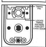
The Digital Exterior Code Pad Assembly is usually factory set for right hand door handing. (The outer knob will turn freely in an anti clockwise direction and resistclockwise turning). To change for a left hand door.
