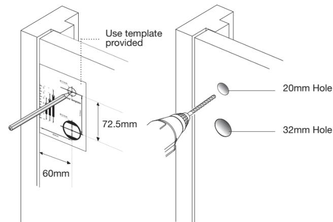
At the height you want your lock, use a pencil to mark a spot exactly 60mm from the edge of the door. At that spot, drill a 32mm diameter hole through the door. Or if using an existing cylinder hole, use the template to mark the position for the 20mm hole.
