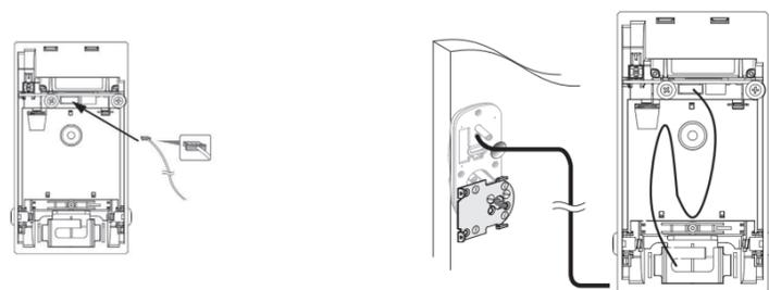
Connect the cable to the battery pack.
