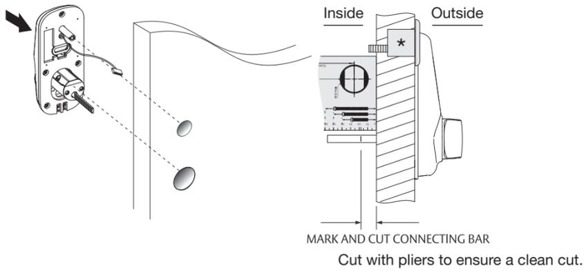
Place the Electronic Keypad into the holes on the outside of the door. Now measure and cut the connecting bar to the required length.
