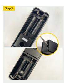
Carefully use a flat head screwdriver to remove both battery covers. Important: Do not install the batteries and operate the External or Internal body prior to installation on the door. This may cause the lock to malfunction.
