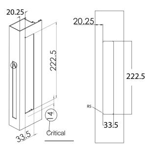
2. Cut holes out for handles on either face of the door, this will be 14mm (critical) above the bottom of lock cut out,
