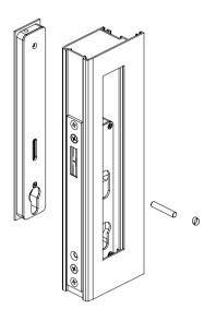
8. Push the euro cylinder lock through lock assembly, Tighten screw to lock cylinder in place.
