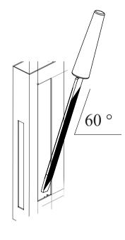
6. Tighten grub screw to lock handles into place.
