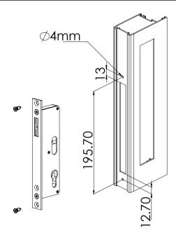
7. Insert Second handle Into frame, following steps 6 and 7 with the driving pin connecting into the Handle.
