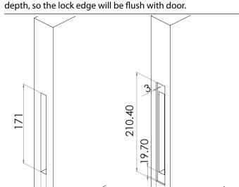
1. Cut out hole for lock in the centre of the stile. (only if stile is symmetrical.) Also cut out hole for lock face plate 3mm
