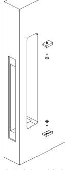
8. Push the euro cylinder lock through lock assembly, Tighten screw to lock cylinder in place.
