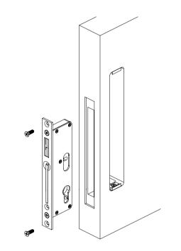
7. Insert Second handle Into frame, following steps 6 and 7 with the driving pin connecting into the Handle.
