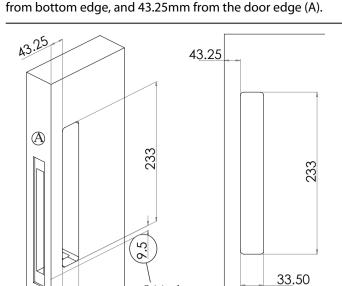
2. Cut holes out for handles on either face of the door, this will be 9.5mm (critical) above the first cut out for the lock
