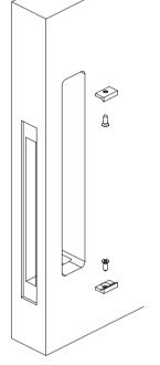
8. Push the euro cylinder lock through lock assembly, Tighten screw to lock cylinder in place.
