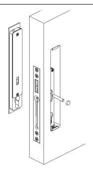
6. Tighten grub screw to lock handles into place.
