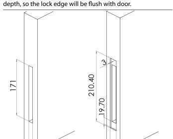
1. Cut out hole for lock in the centre of the stile. (only if stile is symmetrical.) Also cut out hole for lock face plate 3mm
